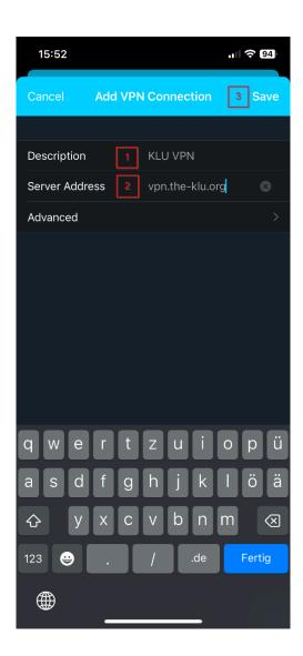
6. After you have pressed "Save" a window will open which you have to confirm with "Allow". After that you will be asked for your device pin/password to take over the VPN settings. Enter your device pin/password
